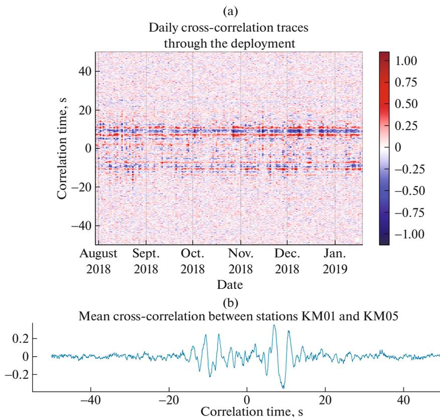
**Fig. 2.** (a) An example of computing cross-correlations for the pair of stations KM01 and KM05 in sliding windows and (b) the result of averaging for the entire observation period.
