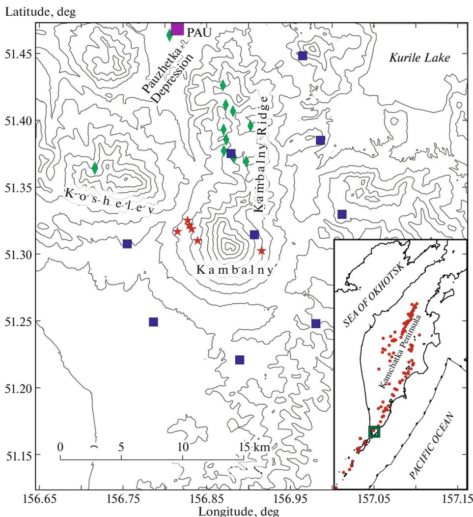
**Fig. 1.** The area around the Kambalny Volcano. The topography is shown by 200-m isolines, the purple square is the permanent Pauzhetka station; and the blue squares show the stations of the temporary network deployed in 2018–2019. Green diamonds are areas of geothermal activity, and red stars are monogenic cones. The inset reflects the position of the research area (green square) and volcanoes of Kamchatka (red dots).
